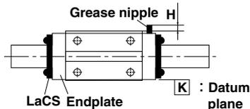
Note: When desiring the mounting location for the grease nipple other than the one indicated in the figure above, contact THK.
