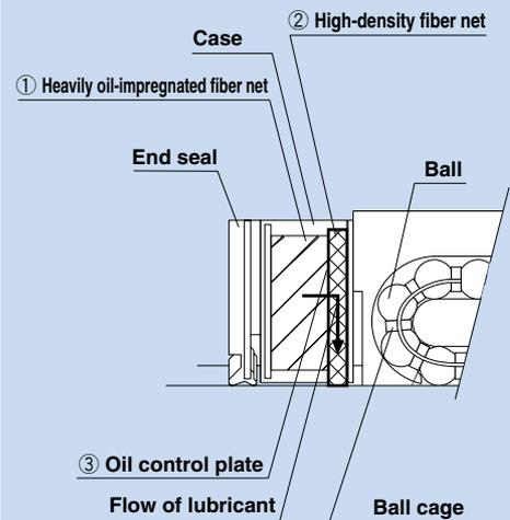
The structure of the QZ Lubricator consists of three major components:
