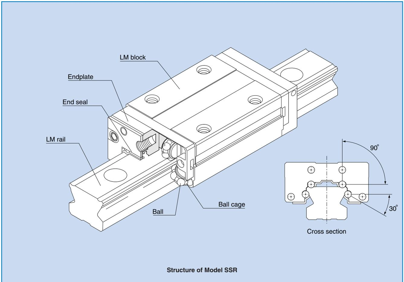
Balls roll in four rows of raceways precision-ground on an LM rail and an LM block, and ball cages and endplates incorporated in the LM block allow the balls to circulate.
